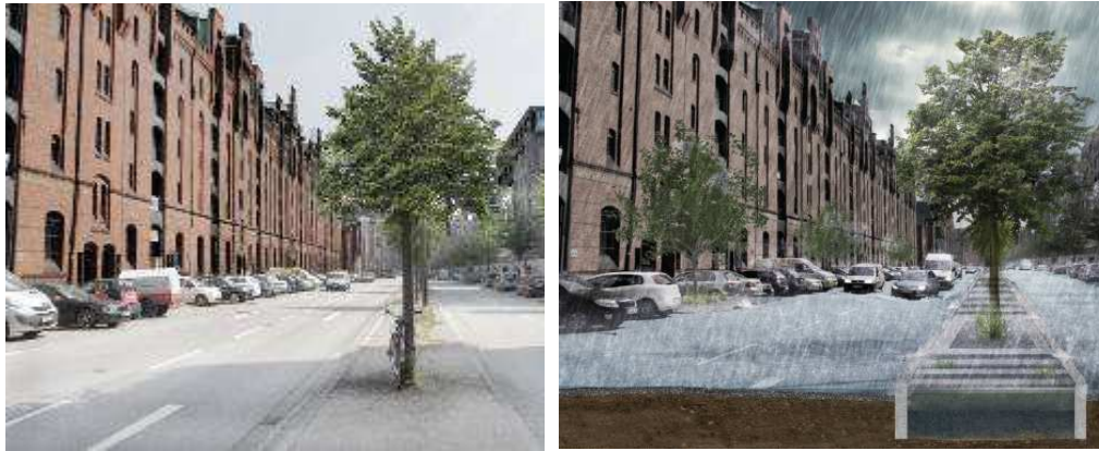
Figure 3: Draft Situation Connecting Road (Left), Water Sensitive Street Space Planning over an absorbent Roadside Tree Grate (right) [FHH 2015]
